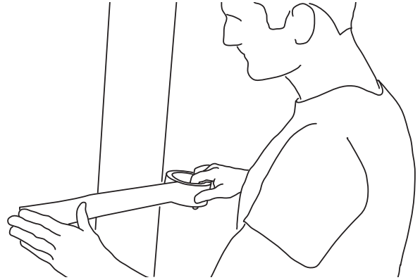
6) We recommend fixing the wall elements with adhesive tape on the back to provide better support.
